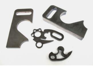
\*ISO 9013 is a standard that defines cut quality of thermally cut parts. The lower the range (range 1 is the lowest), the smaller the angle of the cut face. Cut angle in range 1 is better than in range 5.
